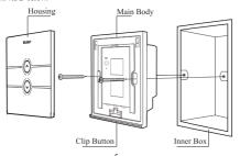
3. Close the housing to finish installation (Join the network before closing the housing).
